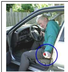
If a person is having difficulty holding the steering wheel, consider a steering wheel knob. A hand brake release and T-bar release enables easier release of the handbrake or the T-bar lever on an automatic transmission.
